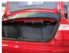
Marine Ply Vehicle Fixing Kit secured under the parcel shelf.
